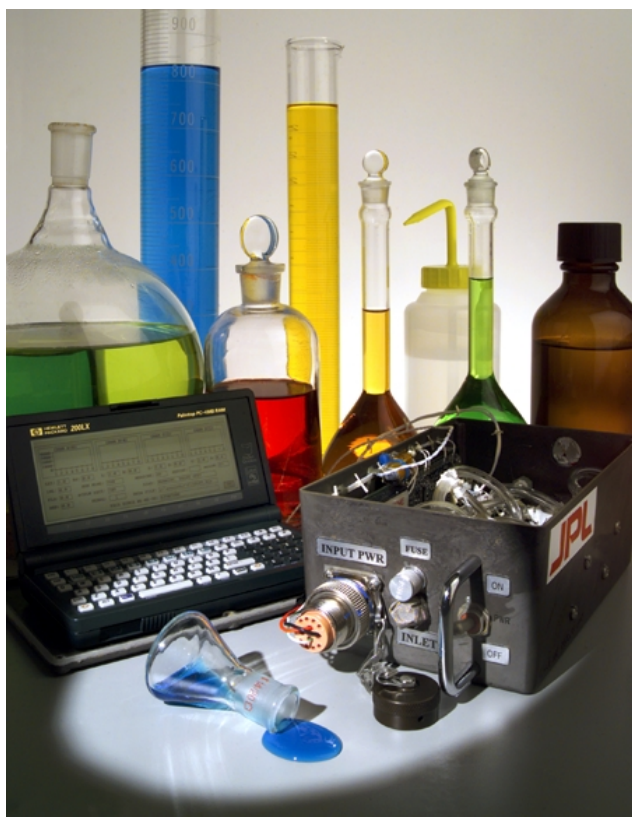
This electronic nose, developed and built at NASA's Jet Propulsion Laboratory, was flown on the Space Shuttle in October 1998.
