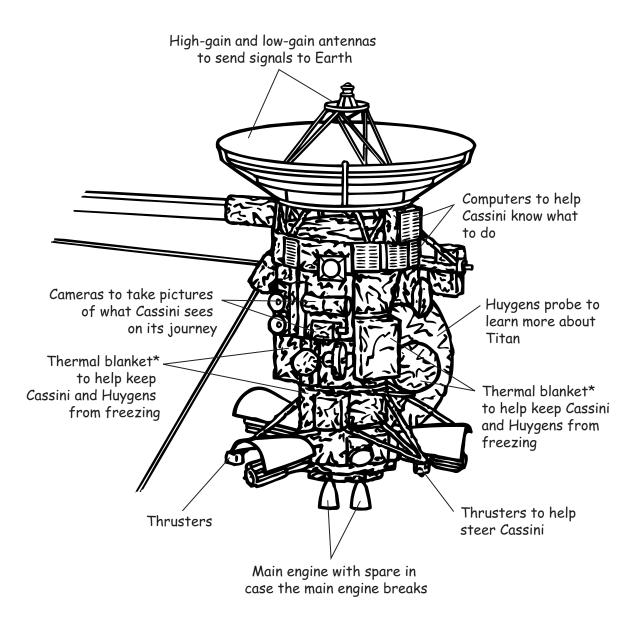
\*The protective thermal blanket is a layered material known as multi-layered insulation or MLI.
