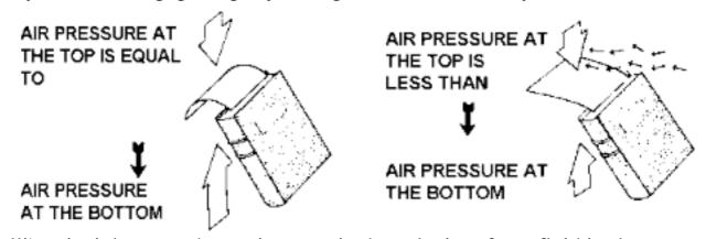
Bernoulli's principle states that an increase in the velocity of any fluid is always accompanied by a decrease in pressure. Air is a fluid. If you can cause the air to move rapidly on one side of a surface, the pressure on that side of the surface is less than that on its other side.
